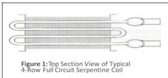
Figure 1: Top Section View of Typical 4-Row Full Circuit Serpentine Coil
