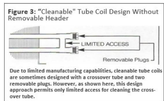
Figure 3: "Cleanable" Tube Coil Design Without Removable Header
