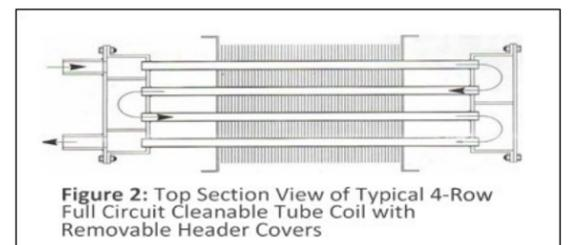
Figure 2: Top Section View of Typical 4-Row Full Circuit Cleanable Tube Coil with Removable Header Covers
